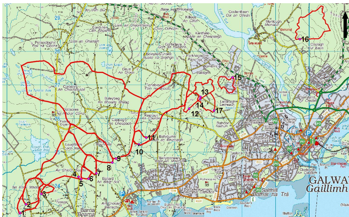
Figure 5 Contributing Catchment Area of Culverts (red polygons)
