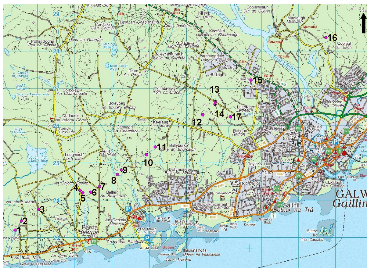
Figure 4 Location Map of Culverts (note reference 11 represents a channel diversion to the northwest of the alignment to achieve a single stream crossing at reference 10)
